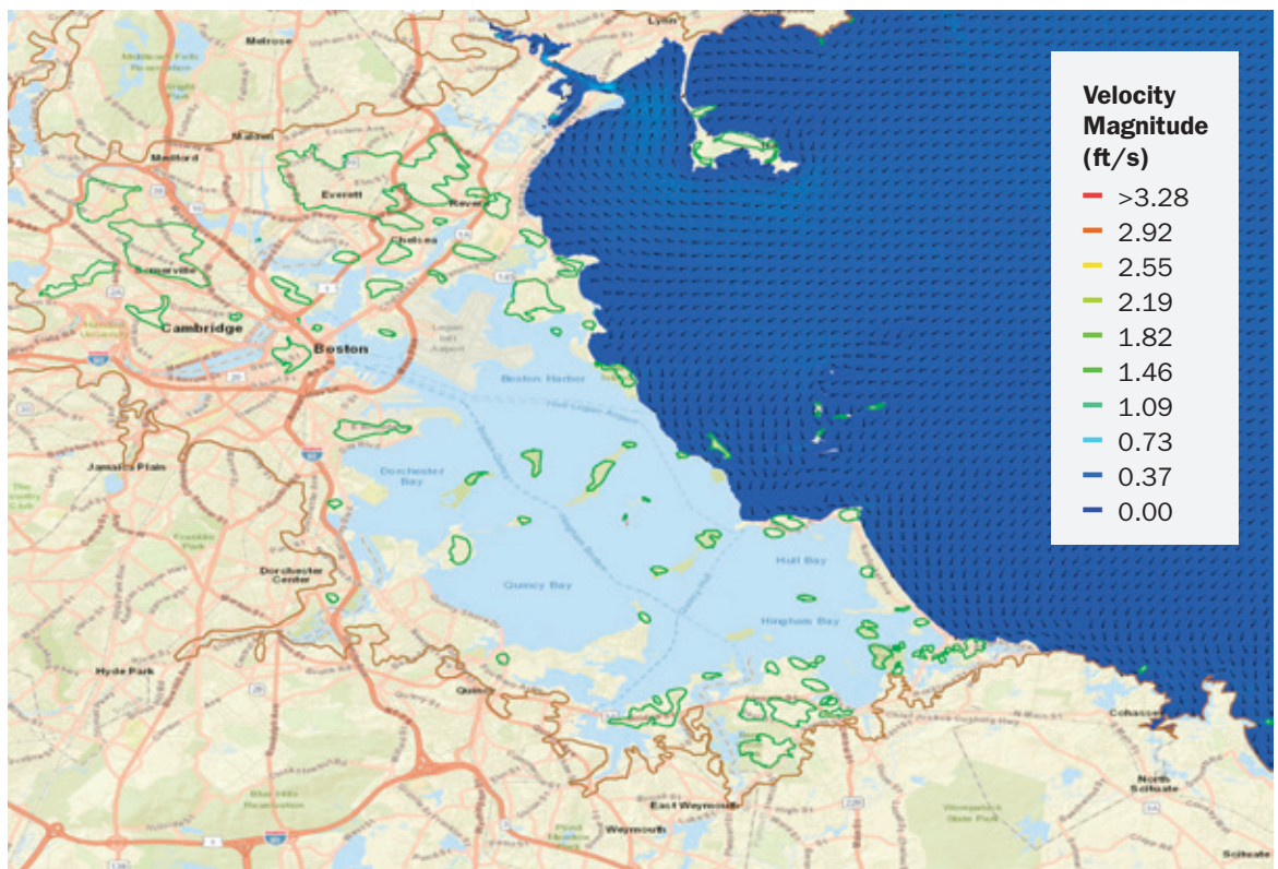
FIGURE 5.15 Circulation with Barrier Closed During Storm
